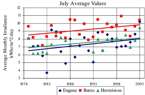
Fig. 4: The trends in average July direct normal values are an example of the increasing summer beam irradiance at Eugene, Burns, and Hermiston, in contrast to the decreasing winter data.
