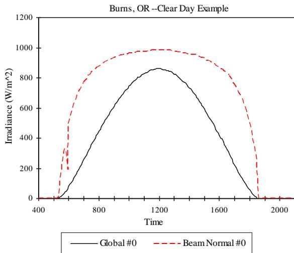
Fig. 7: Example of a clear day graph from Burns OR. These plots were used to identify clear noon periods for the clear day studies.
