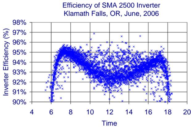
Fig. 7: Efficiency of an SMA 2500 inverter at Klamath Falls, Oregon in June. The data are from 5-minute averaged data.
