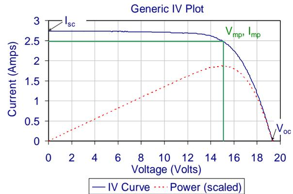
Fig. 2: Generic IV curve for a photovoltaic module. Module power equals current times voltage. The dotted line is the DC power (scaled to fit on plot) plotted for various voltages. The max power point is labeled and can be considered as the rectangle with the largest area that can be obtained using the current and voltage values on the curve.
