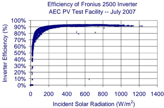
Fig. 3: DC to AC conversion efficiency of a Fronius 2500 inverter plotted against incident solar radiation. The data in the plot comes from the AEC PV Test Facility in July, 2007. The 5-minute AC output power data values are divided by input DC power values.
