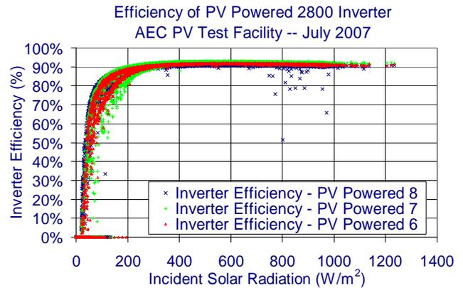
Fig. 4: Efficiency of three PV Powered 2800 inverters plotted against incident solar radiation using 5-minute data. Plot shows the efficiency of turning DC Power into AC Power on July 2007, at the AEC PV Test Facility.
