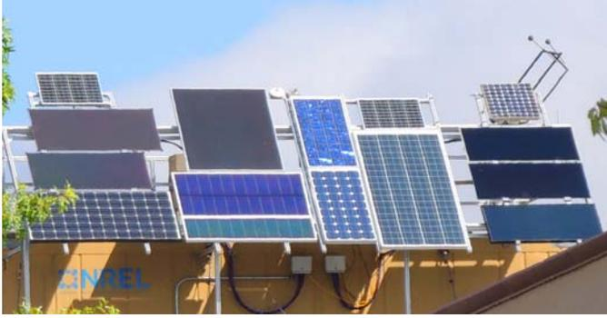
Fig. 1: The NREL PV test facility in Eugene. Picture shot from the lower room and these trees do not shade the modules. The unwashed module is in the upper right hand corner in front of the automatic tracker that can be seen in the background.
