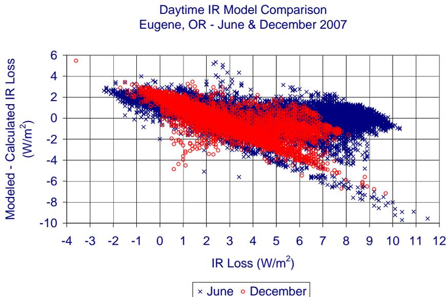
Fig. 5: Plot of modeled minus calculated IR radiative loss plotted against calculated IR radiative loss. The June values are represented by blue x's and the December values are the red circles.
