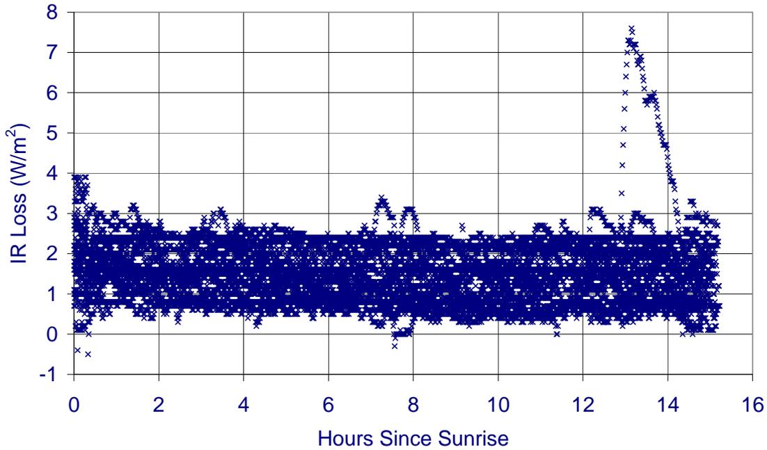
Fig. 1: IR radiative loss values for PSP in Eugene, OR. The spike in IR loss also shows up on other PSPs being monitored at the site.
