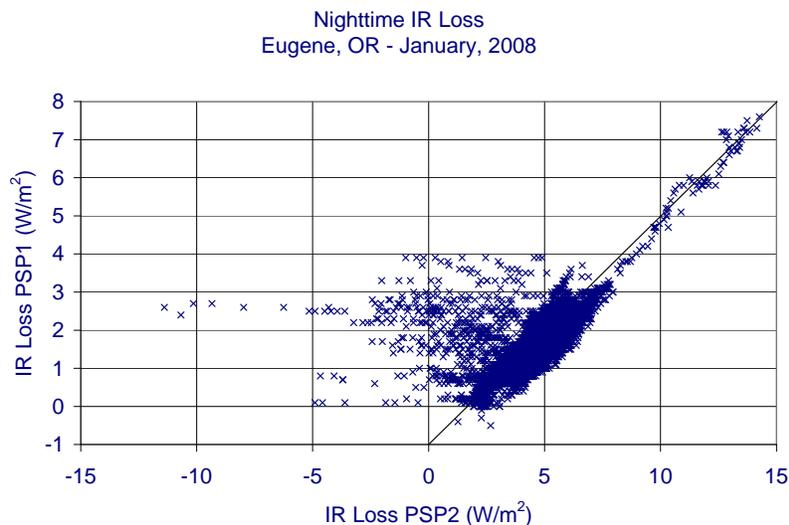
Fig. 8: Plot of IR radiative loss from two different PSP pyranometers at night in January, 2008. Some of the scatter of the points to the left of the main body of points is associated with snowy periods.
