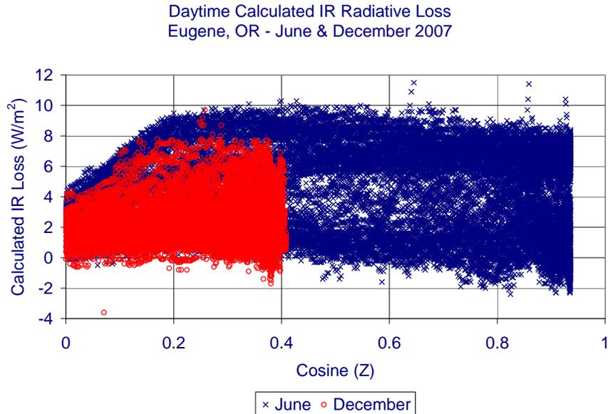
Fig. 7: Plot of IR radiative loss plotted against cosine of the zenith angle. June data points are shown by the blue x's and December data points by the red o's.
