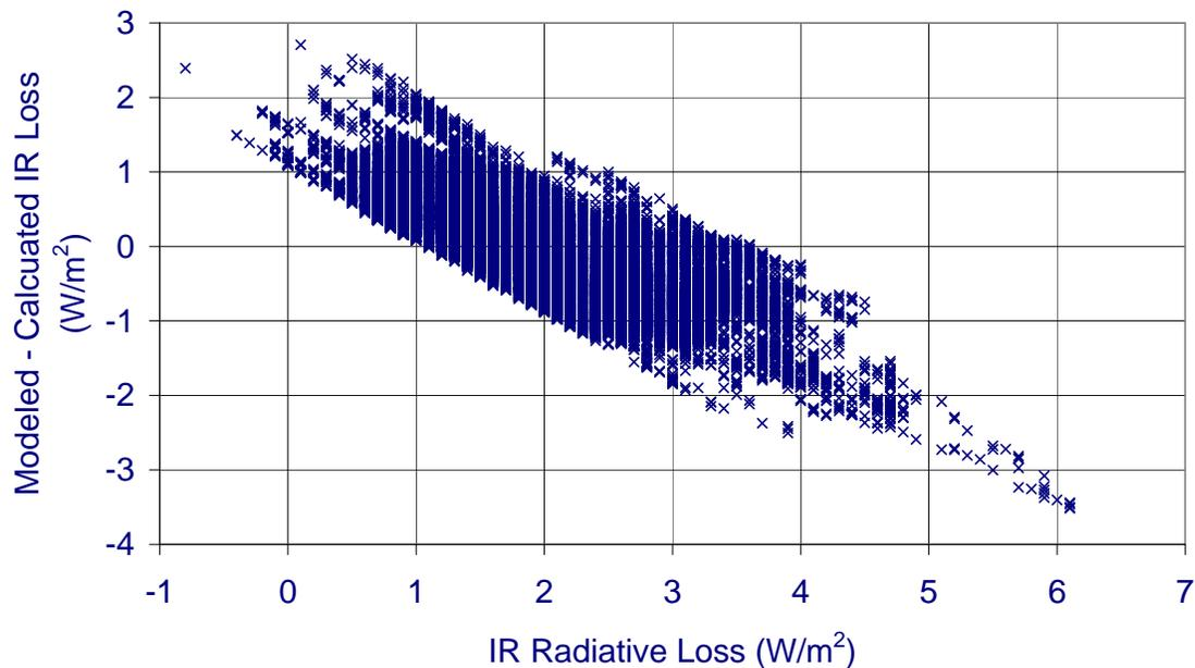
Fig. 2: Plot of the difference between the modeled and calculated IR radiative flux for Eugene, OR. during June and December 2007. Note that the modeled IR values underestimate the high IR values and over estimate the low IR values.
