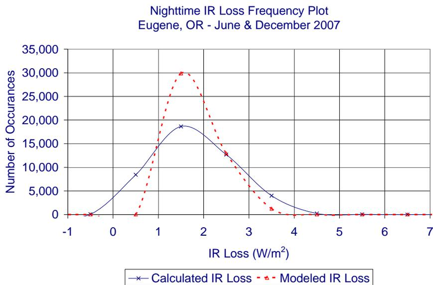
Fig. 3: Histogram of the nighttime IR radiative loss for June and December 2007. Values are binned in 1 W/m<sup>2</sup> intervals.
