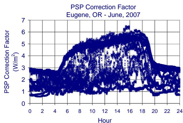
Fig. 1: Calculated PSP Correction Factor using pyrgeometer data. This is a model attempt to calculate the IR radiation from a PSP [1]. 1-minute data.
