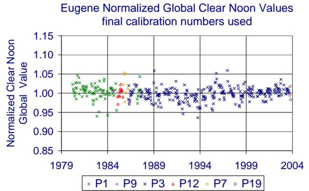
Fig. 8. Plot of clean day solar noon values with the calibration values adjusted on a yearly basis and shown in Figs. 5-7.
