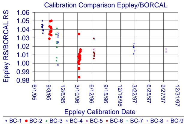
Fig. 3: Comparison of Eppley and NREL calibrations. The large red circles are data from one NREL BORCAL run on June 8, 1996. The two distinct calibration run at Eppley give two distinct distributions.
