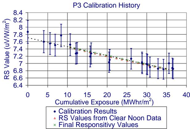
Fig. 7: Calibration history of PSP (“P3”) along with averaged clear day trend, regression fit, and indication of the calibration values used in the database.
