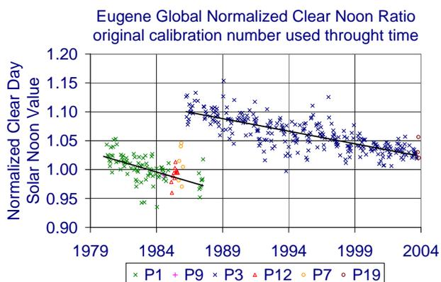
Fig. 4: Clear day solar noon data for Eugene, Oregon from 1980 through 2004. Six different pyranometers were in use during this period. A fixed calibration number was used for each PSP to show rate of change in responsivity.
