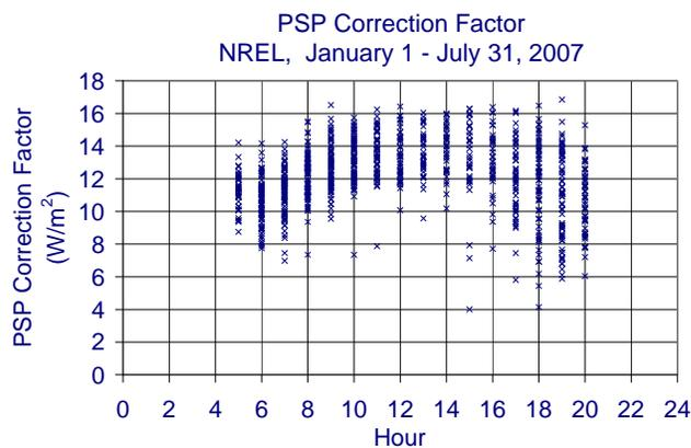
Fig. 2: Calculated PSP Correction Factor using pyrgeometer data at NREL's solar lab. Data courtesy of Ibrahim Reda of NREL.
