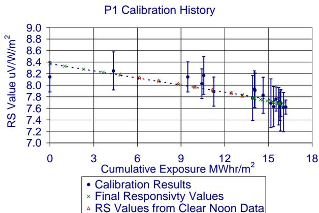
Fig. 5: Calibration record for PSP "P1" plotted over time. The blue dots with the error bars are the various calibrations done over time. The red triangles are the clear day trend. The green x's are the actual responsivity values used.
