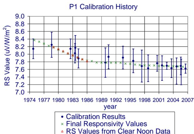
Fig. 6: Same data as plotted in Fig. 5 except plotted against time. In 1987, the pyranometer was removed from daily operation and was used as a reference instrument.
