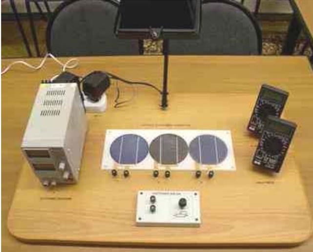
Fig.10. Prototype PV lab kit developed by Igor Tyukhov. This design served as the basis for the UO SRML PV kit.
