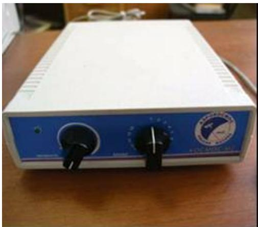
Fig. 1: Receiver for satellite images
