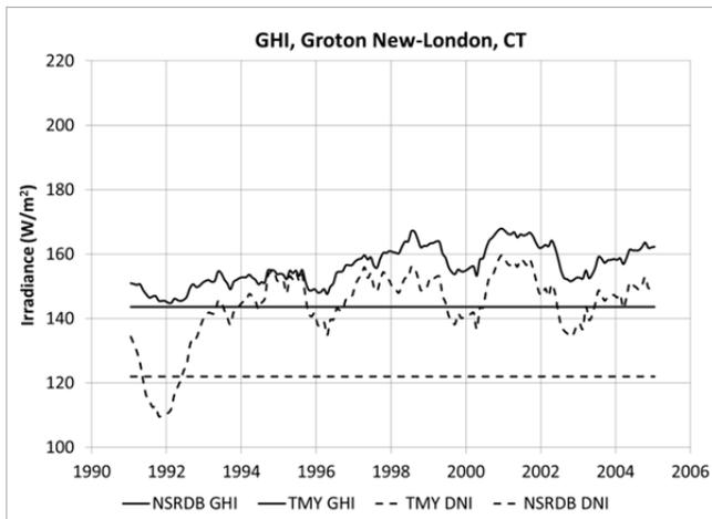
Fig. 1: Plot of GHI and DNI for Groton-New London, CT. The straight solid line is annual average GHI from the TMY3 data file and solid line is the annual average GHI from the NSRDB data file. The dashed straight line is the annual average DNI from the TMY3 file and the dashed curved line is the annual average DNI from the NSDB file.
