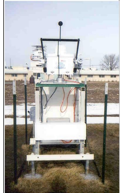
*Solar monitoring equipment mounted on an automatic tracker at Twin Falls, Idaho.*
