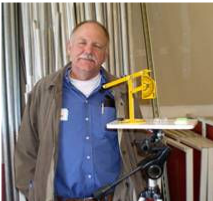
Fig. 3: Scott Sayles shows off his site analysis equipment. He built this using designed from an OSU Extension Service newsletter for $29 in parts (two protractors, compass, and level) plus a tripod.
