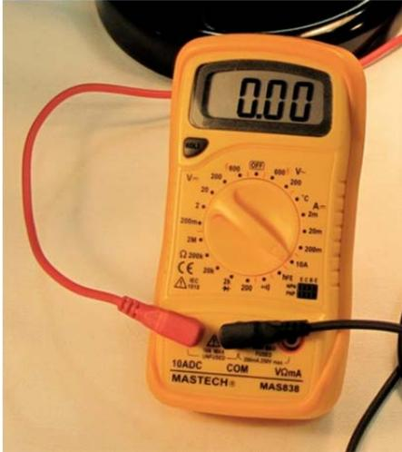
Fig. 1: Multimeter as Ammeter
