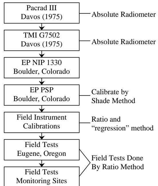
Fig. 6. Flow diagram showing the absolute calibration process.
