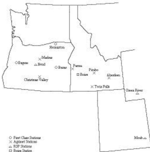
Fig. 1: UO Solar Monitoring Network. Open circles (○) indicate stations containing both global and beam solar instrumentation. AgriMet stations are labeled (X). Global and diffuse irradiance are measured at AgriMet stations. Triangles (△) show the location of RSP stations. RSP stations measure global and diffuse radiation and calculate beam radiation. The Boise station has both an RSP and AgriMet instrumentation and is labeled with a square (◻).
